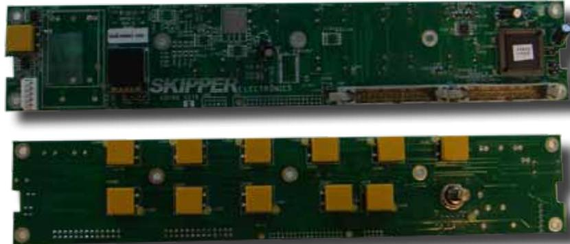
**The PK-C001 is a PCB keyboard for the SKIPPER DL850/EML224 Navigational Speed Log.**
